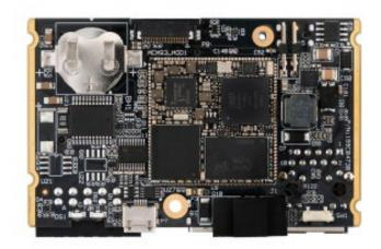
SBC-IOT-LINK-iMX93 is an Internet of Things (IOT) Single Board Computer based on the NXP i.MX93 processor designed for industrial control and monitoring.
